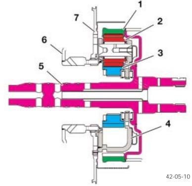
Lepelletier Planetary Gear Train
